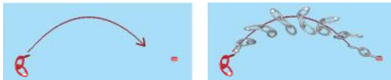
Fig. 12. A sketch of the chain motion is converted automatically into a physical motion of a chain flying across and reaching the red box with a white ball. The chain is modeled as a series of three rigid links connected by two universal joints.
