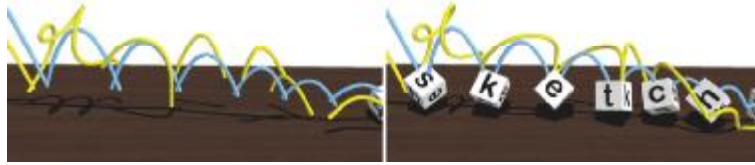
Fig. 9. On the left, the sketched trajectories of the center of mass (blue curve) and the die corner (yellow curve) are discontinuous. The figure illustrates the gaps in position and orientation at each collision. Gaps in velocities also exist but are not illustrated in the figure. On the right, parameter estimation removes the gaps in position and orientation to create continuous motion trajectories. Velocity gaps are also reduced but cannot be eliminated completely because the task is overconstrained.
